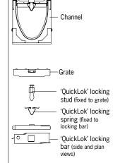
ACO 'QuickLok' is a patented boltless locking system, grates are removed and replaced with the minimum time and effort for ease of maintenance. The unique design provides a positive 'snap down' fit into the locking bar. A stud is fixed to the grate which 'locks' into the spring clip in the locking bar.
